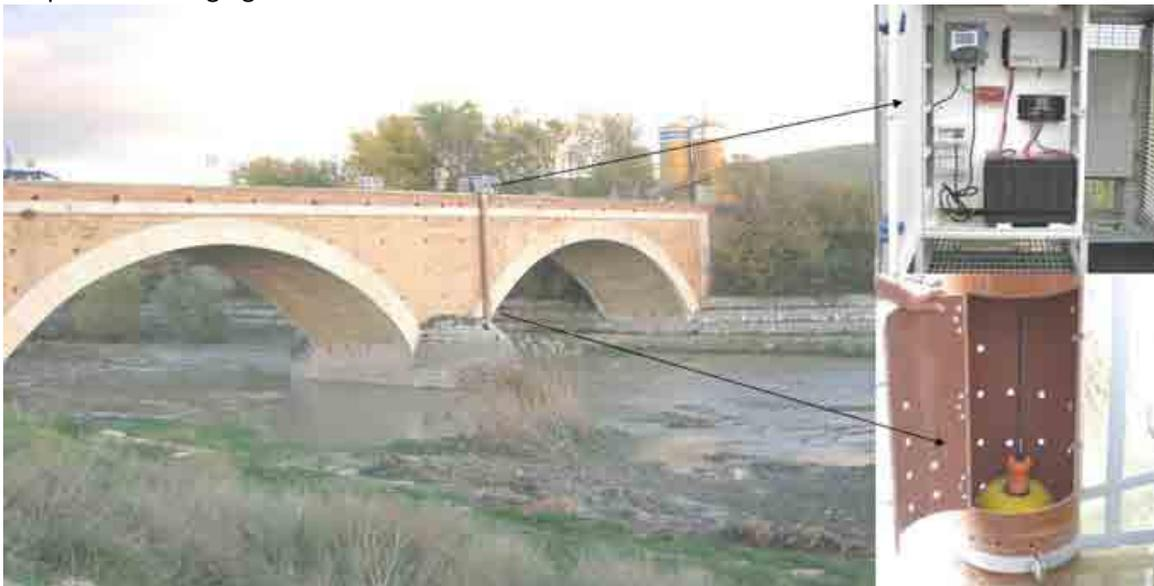
Figure 2. Sediment transport measuring station, optical probe housing (right, below) and data acquisition system (right, above).
