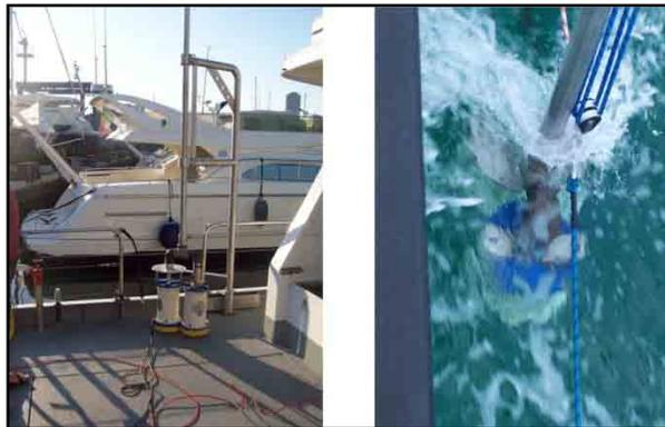
*Figure 1. Two ADCP at different frequencies installation and in action.*
