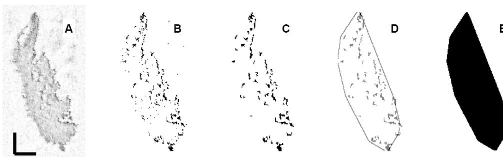
Figure 4 Processing sequence for projected area estimation (E) from in-focus particle image (A).
