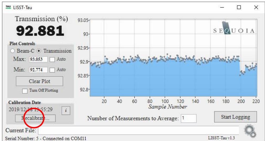
The instrument can be recalibrated through an automated procedure by selecting the recalibrate button. See *Clean-water Baseline Measurement (Calibration)* on page 14 for more information on this process. If you proceed with recalibrating the instrument you will be asked to confirm the new calibration coefficients. **The previous calibration coefficients will be overwritten and are not recoverable!**
