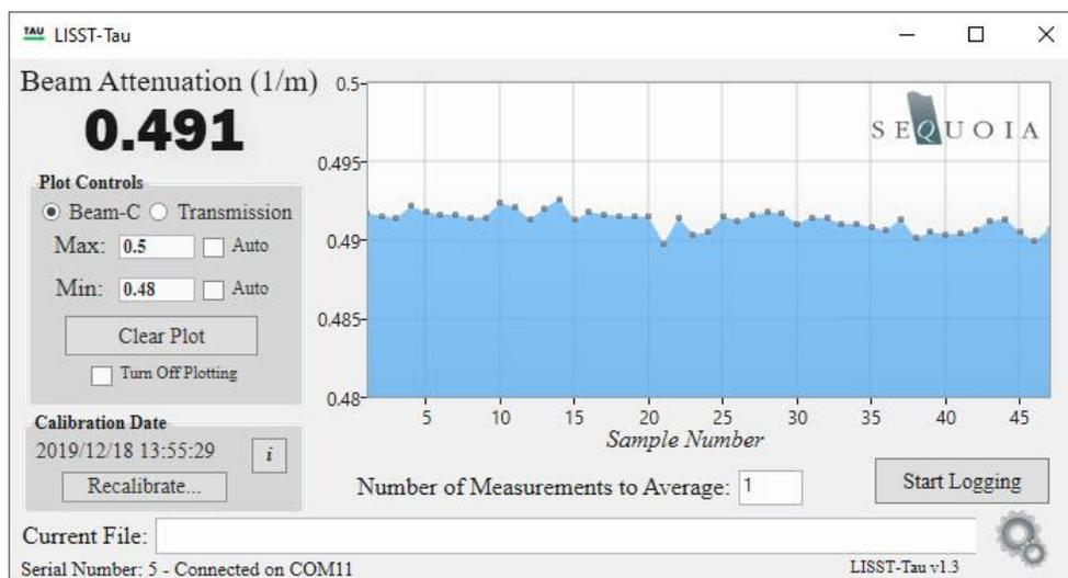
In the 'Plot Controls' group box, you can customize the scale of the current plot, clear out the existing data, or turn off plotting all together. Turning off the plotting option may be useful if computer resources are limited.
