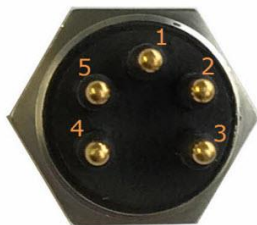
Power-communication connector SubConn MCBH5M
