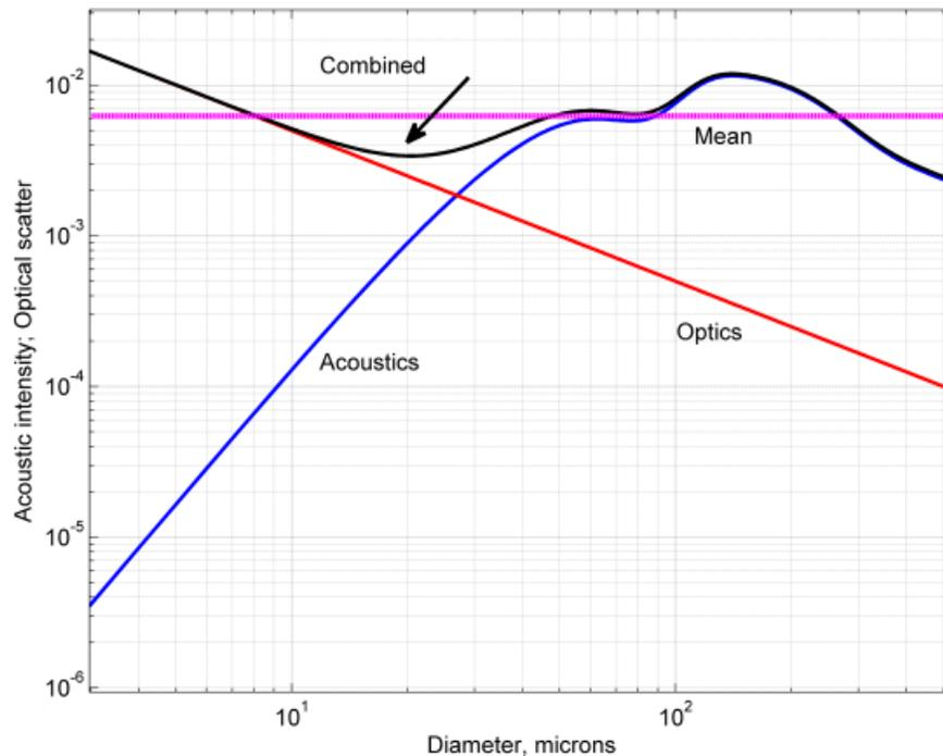
Figure 1—ABS and OBS response versus particle size
