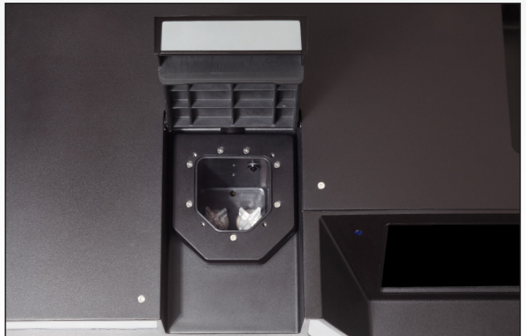
Top view: open chamber with mixers
