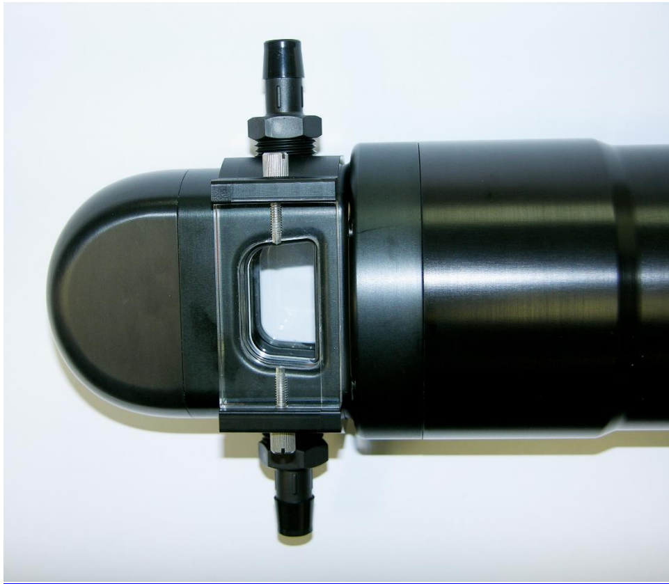
Full Path Flow Through Chamber for LISST-200X
