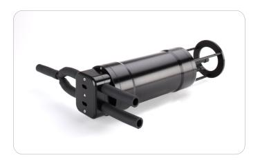
The FlowControl-Sub typically profiles unfiltered water on down casts and filtered water on up casts. An on-board data logger monitors the depth and switches to filtered water on the up cast. The filtered and unfiltered measurements allows for differential measurements of particle properties from a single cast, saving time and resulting in higher quality profiles in highly variable waters..
