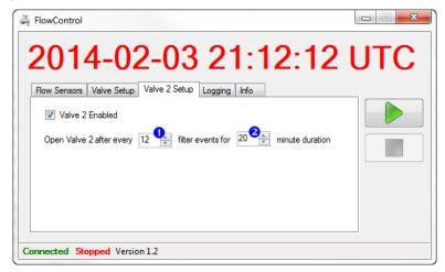
Valve 2 will open after every specified number ① of filter events, for a specified duration ②. For example, the figure below shows the system state (0=total, 1=filtered, 2=valve2 open) for half-hourly events, 10 minute filtered duration, with 10 minute valve 2 duration every 4 filter events.
