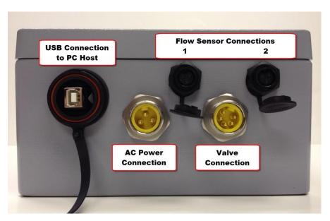
Connect dust caps to prevent seawater, dirt, or other contaminants from damaging connectors when not in use.
