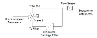
Instruments are either arranged to be fed in parallel by a manifold such that flow can be varied independently for each, or the instruments can be arranged
