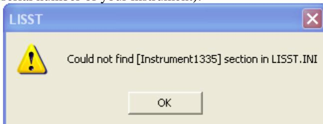
**A:** Go to your C:\WINDOWS folder and search for the LISST.INI file. Open it up in Notepad or a similar text editor. Make sure that the section containing your instrument calibration constants are located in the file. If not, copy them from the LISST.INI file that was included on the ship disk for your instrument. Then re-save the edited LISST.INI file in C:\WINDOWS.
