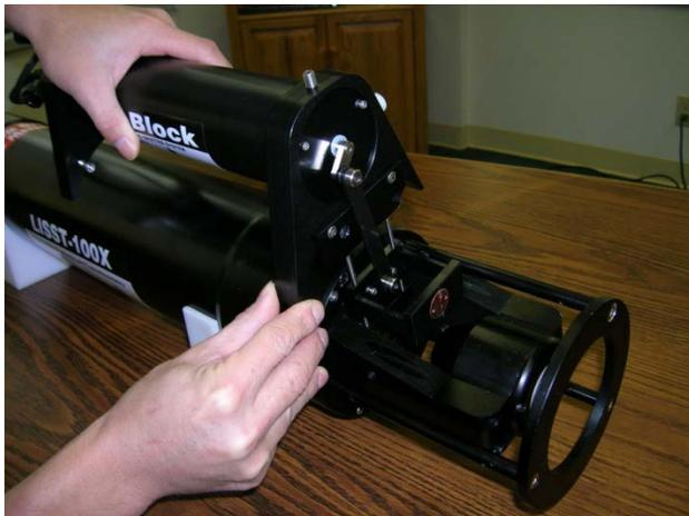
the Closed position to facilitate re-installing it at a later date. The BioBlock may be commanded to go to the Closed position prior to installation by connecting it to the LISST-100X and using the LISST-100X software. Do not manually rotate the crank arm that drives the shutter.
