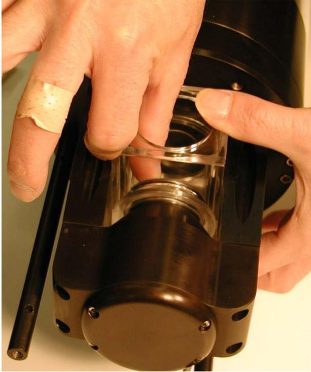
**Step 1)** Before installing the Small Volume Horizontal Chamber first clean the windows of the LISST-100X. On older versions of the LISST-100X it will also be necessary to remove the endcap ring and standoffs on the optics endcap. Remove the three screws on the ring and then unscrew the standoffs. Remove the Spacer and push the Slider into toward the center of the chamber.
