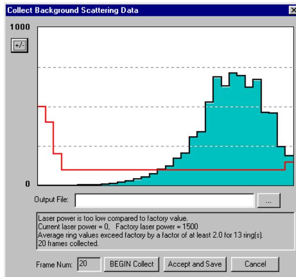
When the *BEGIN Collect* button is pressed 20 samples will be displayed to the screen as they are acquired. After all 20 are collected the average will be displayed. If the values are acceptable the values can be saved to a file. Enter the filename in the box and press the *Accept and Save* button.
