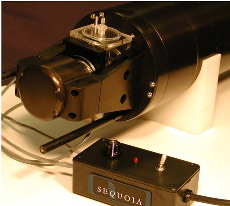
**Step 4)** The chamber can now be filled with clean water. It is highly recommended to do a background scatterfile after assembly to make sure that the windows are still clean. It is NOT necessary to have water around the chamber; only IN the chamber.
