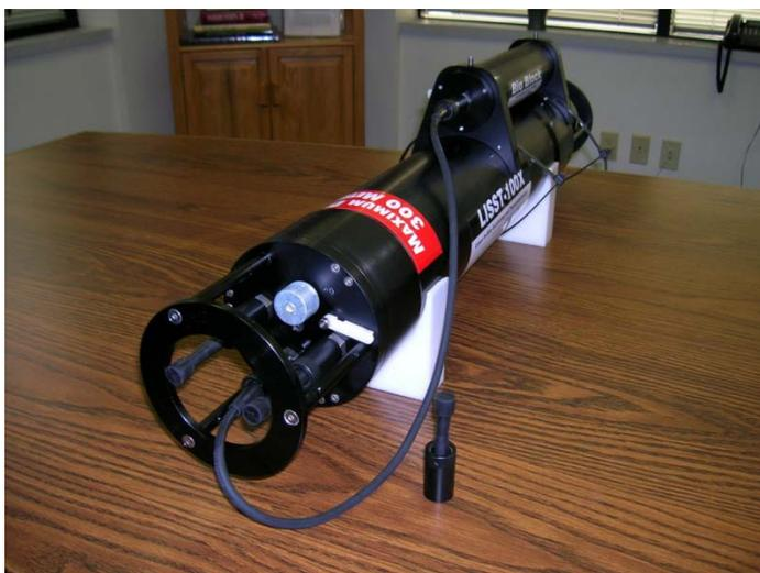
**Step 5)** Connect the BioBlock cable to the LISST-100X. Verify normal operation by cycling the system using the LISST.EXE software. The BioBlock shutter should position itself smoothly during cycling, with no binding. If necessary, loosen the mounting screw slightly and adjust the position of the BioBlock slightly to improve operation, and then re-tighten the screw.
