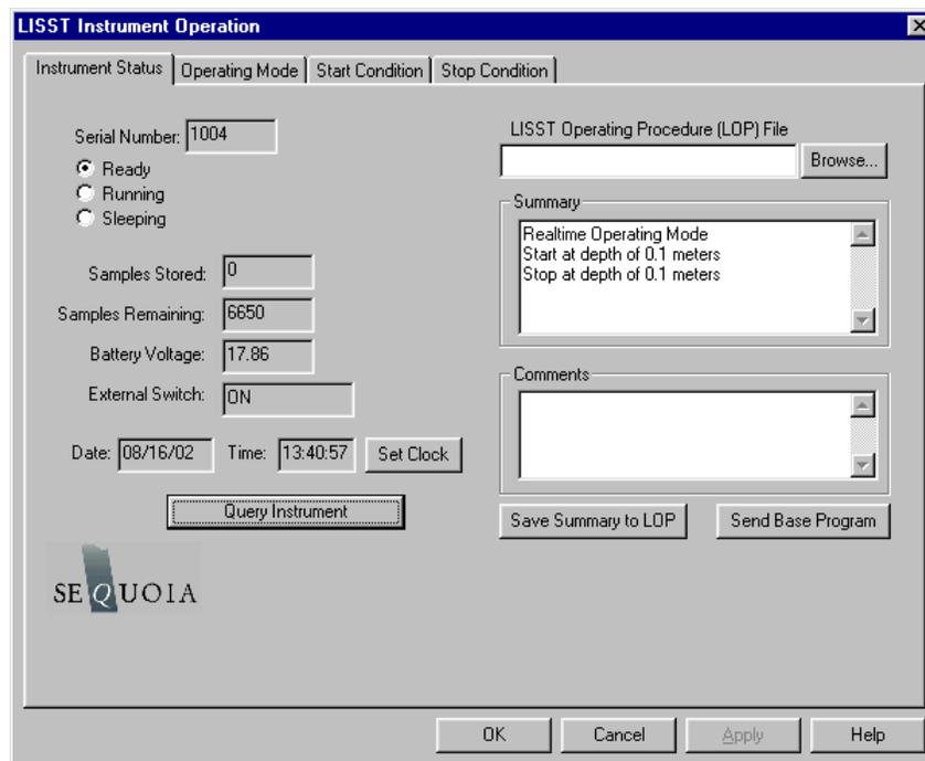
The window has four tabs, Instrument Status, Operating Mode, Start Condition, and Stop Condition. The Instrument Status page gives information about the current instrument. It also allows previously saved instrument configuration files to be loaded on to the instrument. The ability to save the current settings to a file is also available. The Summary window shows the current deployment configuration.
