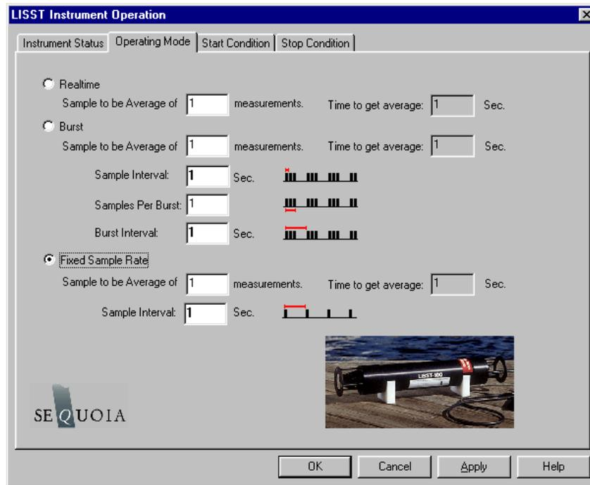
The RealTime mode is used for real-time size distribution displays. This mode sends the raw data to the LISST-SOP software for conversion to Size Distribution and displaying on the screen. No data is saved in the datafile when this mode is used.
