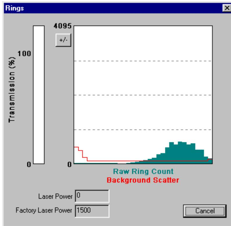
The view rings display is also available when processing a Raw Data file. However, it is not available when viewing a processed Size Distribution file.
