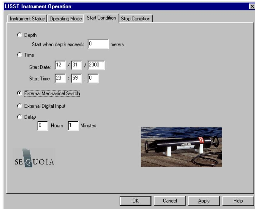
There are five options: Depth, Time, External Mechanical Switch, External Digital Input, and Time Delay. Select the mode by clicking on the button next to its label. Select the correct parameters as required. For this example let's select the External Mechanical Switch Start Condition.
