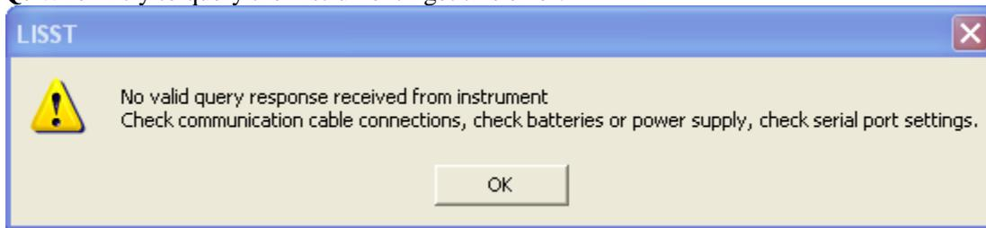
**A:** In addition to checking the cable, power and serial port settings, make sure that the instrument is not running. Open up the terminal window and confirm that no program is running. If a program is running, stop it by clicking the stop button, close the terminal window and try to query the instrument again.
