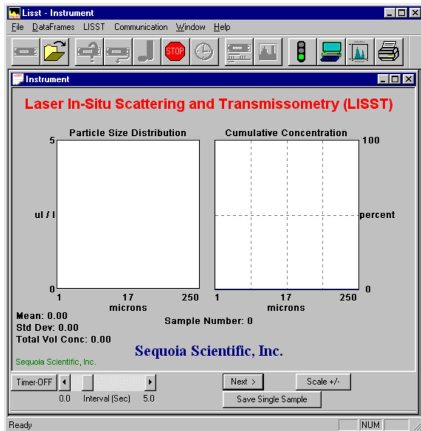
Use the Timer button to start and stop data collection. The slider bar controls the data acquisition time.
