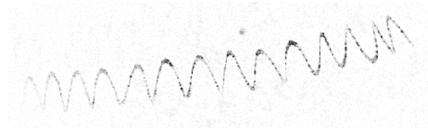
Two reconstructed images from the LISST-HOLO that show features that are only 2-3 pixels wide (10-15 microns).
