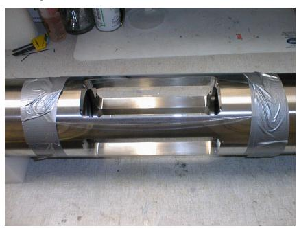
The instrument should be placed horizontally on the supplied white plastic supports. Roughly 2 liters of water is needed to do a ZSCAT.
