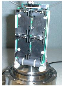
The LISST-Deep should not require any adjustment or calibrations. The pressure and temperature sensors can be recalibrated if desired. The performance of the instrument can be checked with the use of a sample of particles of a known size distribution.
