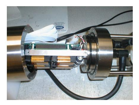
The batteries are held in standard holders. Remove the batteries and replace with new. To increase battery capacity the alkaline batteries can be replaced with lithium 9V batteries. The battery holders are shown below.
