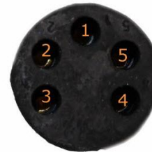
Mating cable connector SubConn MCIL5F
