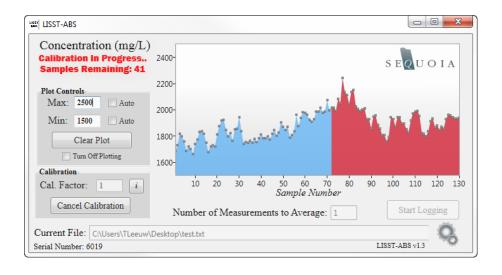
The sample number will count down from 100. Once completed, a new calibration factor will be calculated and entered into the text box. This calibration factor will be saved in the software between sessions (i.e. next time you open the software, 'Cal. Factor' from your previous session will be filled in automatically).
