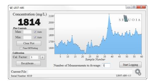
If the Sequoia USB cable is not available you can still use the software via any RS232 connection to the PC. You will need to power the instrument separately. See Appendix A for wiring instructions.
