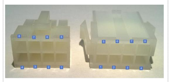
The long cable is terminated with a Molex Mini-Fit Jr Female connector (Molex # 0039012081 with Molex # 0039000431 pins). The mating pigtail cables use a male connector with a latch (Molex 0039012080 with Molex #0039000073 sockets). Both connector have labels for the pin numbering molded into the plastic body of the connector. The pin number is also shown above.
