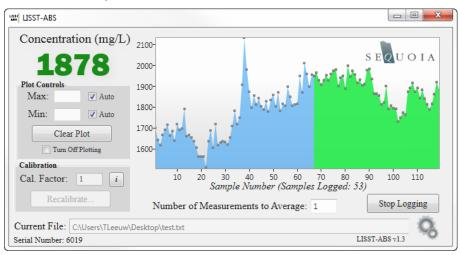
The log file header contains calibration information, the computers current time zone, and the instrument serial number. The header is followed by three columns of data: date, time, and concentration (mg/L).
