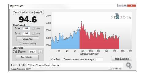
If you elected to save the uncalibrated ABS values, a text file will be saved at the location you specified before starting the calibration. It will contain a header with calibration information, followed by the 100 uncalibrated ABS measurements used to calculate the new calibration factor.
