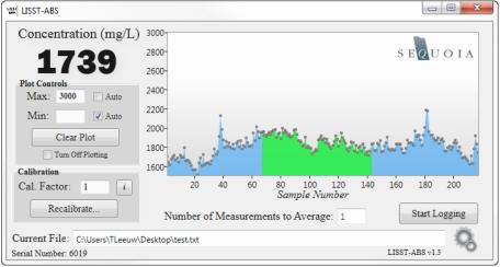
The data currently in the plot can be cleared by pressing the 'Clear Plot' button. This will only clear the display and will have no effect on data logging or calibration. If the software is left to run for a long period of time, the plot will show a maximum of 900 data points (15 minutes at a measurement average of 1). After 900 points, the x-axis will scroll, showing only the most recent 900 points.
