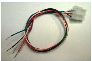
The wires are labeled and color coded. Connect the Black wire to Power Ground. Connect the Red wire to +12V. Connect the Green wire to Analog input and the White wire to the Signal Ground.
