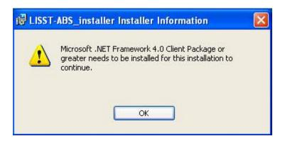
Should you receive this message, return to the ship disk and run the 'dotNetFx40\_Client.exe' installer. This will install the .NET framework on your computer. Once that is completed, relaunch the 'LISST-ABS\_installer.exe' and follow the installation instructions. The installer will place a LISST-ABS shortcut on your start menu as well as your desktop.
