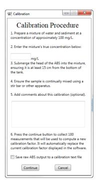
The concentration displayed in the software will be incorrect until an accurate calibration factor is entered in the software (see Appendix B for an explanation of calibration constants). If you are only interested in viewing and logging uncalibrated concentration, you can skip this section.
