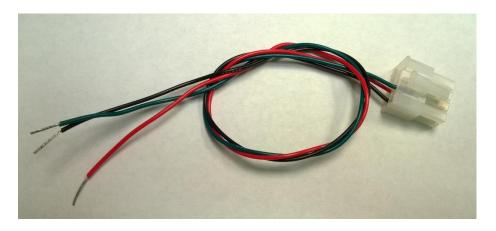
The wires are labeled and color coded. Connect the Black wire to Ground. Connect the Red wire to +12V. Connect the Green wire to SDI-12 Data.
