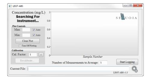
Ensure the instrument is connected to the computer via the USB cable. Within a few seconds the software will find the instrument and begin displaying uncalibrated concentration values (default calibration factor of 1). The instrument serial number will also be displayed at the bottom left of the screen. The software will automatically start plotting the uncalibrated concentration as function of sample number.
