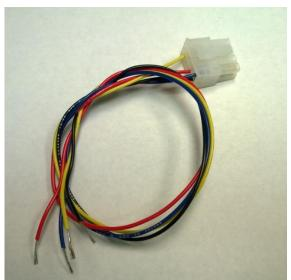
The wires are labeled and color coded. Connect the Black wire to Ground. Connect the Red wire to +12V. Connect the Yellow ABS Transmit wire to the datalogger Receive input and the Blue ABS Receive wire to the datalogger transmit output.
