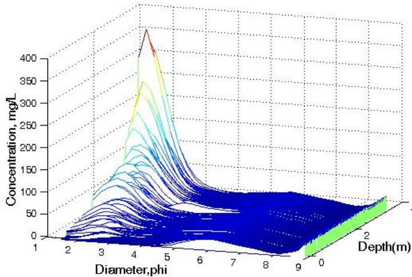
Figure 5: Size Distribution of suspended particles in a vertical profile displays a constant mode a phi value of about 5, and a rising mode with depth, centered around a phi value of 1.
