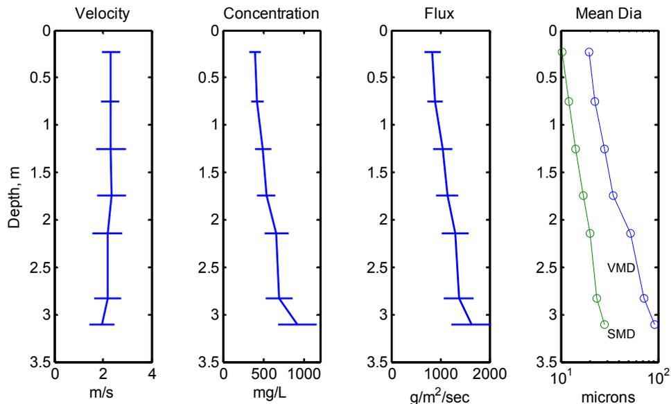
Figure 6: Mean  $\pm$  one standard deviation of the profile. Note SMD is magnified 5x. Note also, the logarithmic size scale in the last panel.
