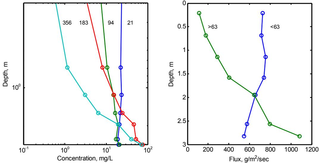
Figure 8: (left) concentration profile of 4 different particle sizes (numbers are sizes in microns; note the well-mixed 21 μm size mode) ; and (right) flux of fine (<63 vs coarse (>63 microns).
