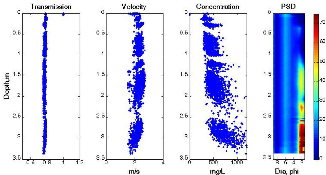
Figure 4: The raw recorded data in one profile. In the optical transmission profile, clear water background calibration points are seen at the surface with transmission of 1.0, and corresponding concentration of 0 is visible at the top of the concentration profile.
