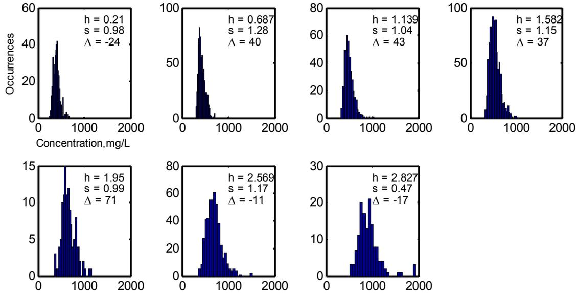
Figure 7: Histograms of sediment concentration, depths 0.5:0.5:3.5m (left to right, top to bottom). Depth is shown as h (m), and the skewness of each distribution is shown as s on each plot. The bias, i.e. difference of mean and most frequent occurrence is shown as Δ mg/L
