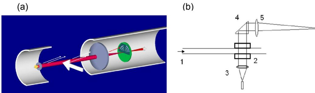
Figure 1: (a) Optics of laser diffraction, simplified, (b) actual in the LISST-SL; 1- water intake; 2 – optical windows; 3 – collimating lens; 4- laser folding prism; 5 – focusing lens.
