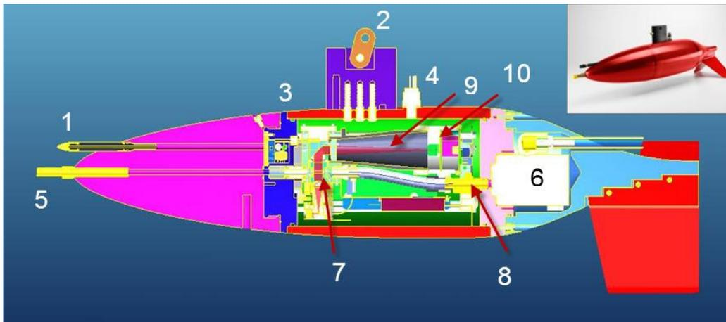
Figure 2: The LISST-SL instrument in cross-section. 1: pitot tube; 2- lifting point, 3- static port; 4 underwater connector; 5- water intake; 6- intake assist pump; and 7 – laser beam at measurement volume; 8- temp sensor; 9- scattered light path; and 10- ring detector (seen edge-on).
