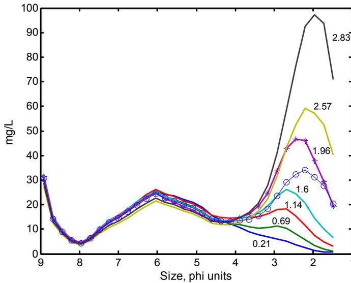
Figure 9: The mean PSD's at all 7 depths (solid lines); the profile-mean PSD (-o-), and the PSD at half-depth (-\*-). Numbers on curves are depth in m.
