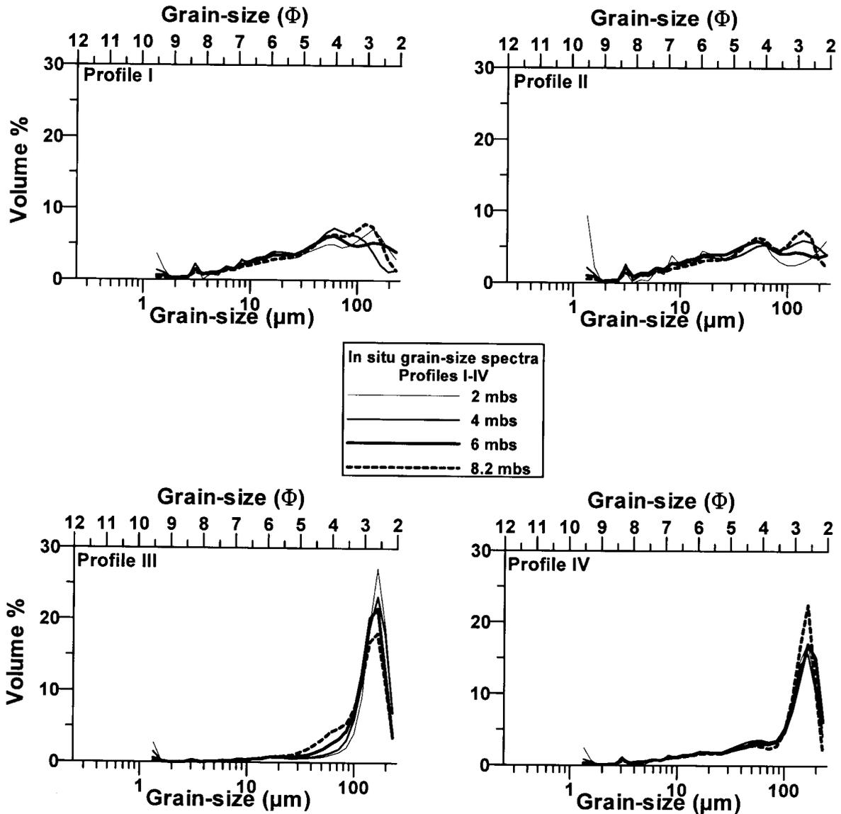
Fig. 3. In situ grain-size spectra at 2, 4, 6 and 8.2 mbs in the four profiles. Note the disappearance of particles smaller than  $4 \Phi$  ( $64 \mu\text{m}$ ) in profile III and IV compared to profile I and II.
