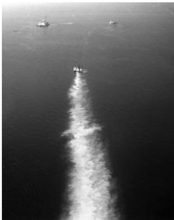
Fig. 2. Photograph of a typical dredging plume in the Øresund. Current direction is towards the North (bottom of photograph). Note the sharply demarcated edges of the plume. (Photo by Poul Hammer, Danish Hydraulic Institute.)
