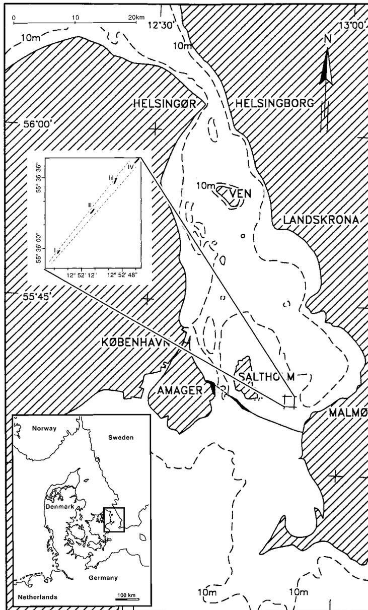
Fig. 1. Map of the Øresund area between Denmark and Sweden. Inset shows the position of the profiles (I–IV) in the investigated dredging plume. The position of the dredger was approximately 300 m SW of profile I. The edges of the plume are indicated by the dashed lines.
