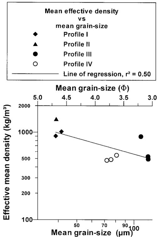
Fig. 6. Plot of effective density versus in situ particle size in the four profiles. The effective mean density is generally seen to decrease with: (1) increasing mean grain-size, and (2) from profile I/II to III/IV.
