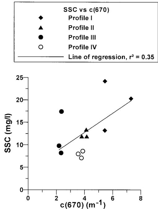
Fig. 7. Scatterplot showing the correlation between SSC and  $c(670)$  for the water samples taken in the profiles. Almost no correlation between SSC and  $c(670)$  is seen.
