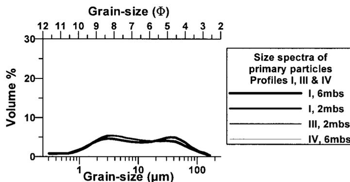
Fig. 4. Selected grain-size spectra of the primary particles in the profiles. Note the similarity of the spectra, when compared to the large difference in the in situ spectra in Fig. 2.
