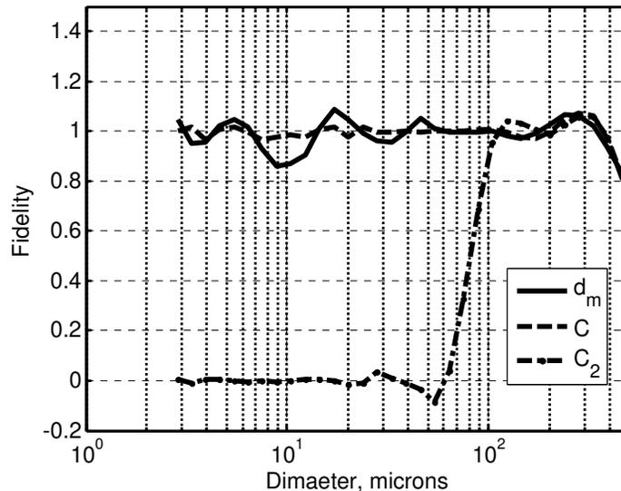
Fig. 4. Numerical simulations: Fidelity testing of weight functions for estimating mean diameter, total, and sub-range concentrations. (The ordinate is fidelity).
