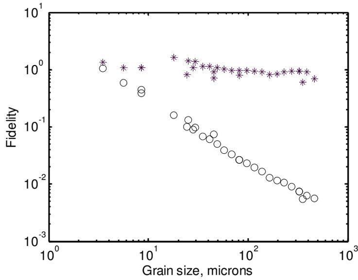
Fig. 5. Fidelity of measurement of concentration of random shaped natural grains. The weighted sum (\*) shows a near constant value. In contrast, an optical transmission-based estimate (o) shows essentially  $1/d$  dependence, producing a 2-order of magnitude variation in calibration.
