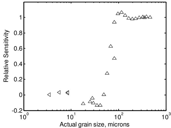
Fig. 7. Effectiveness of the coarse-particle sensor weight factors  $\underline{T}_{v,2}$ . This relative sensitivity to particles of different sizes closely mirrors the theoretical response of Fig. 4.
