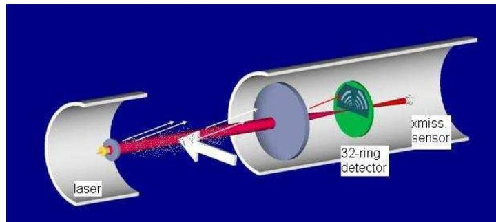
Fig. 1. Schematic of a laser diffraction set up, showing *left to right*, a collimated beam, a receiving lens, and a set of ring detectors in the focal plane of a receiving lens.
