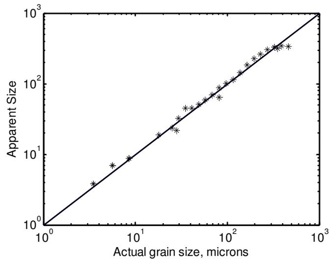
Fig. 6. Fidelity of estimation of mean diameter (\*). The straight line is 1:1.
